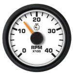
This 2-inch Tachometer connects to the Magnetic Pick-up sensor. The tachometer has four range selections for rough calibration and an adjustment potentiometer for fine adjustment.
