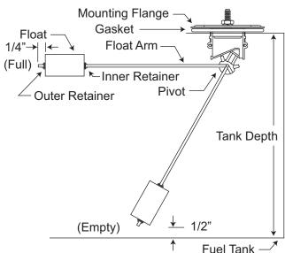
3. Slide the Float and both Retainers toward the Pivot along the Float Arm to the desired length. Leave about 1/4 inch of the arm beyond the Outer Retainer and cut off the excess. Do not position the Inner Retainer at this
